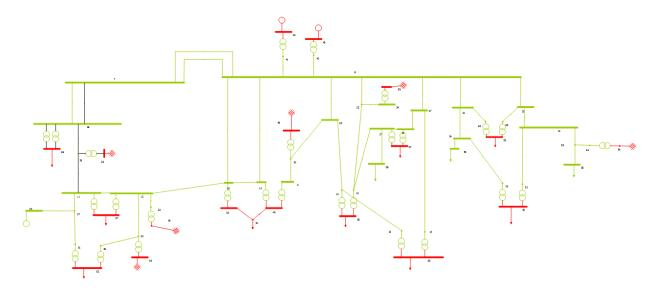
Figure 1 High voltage network model of IoW in IPSA2
