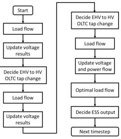
Figure 1 Flow chart of the control scheme
